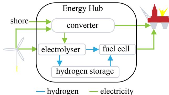
Figure1: Conceptual illustration of offshore energy hubs.
