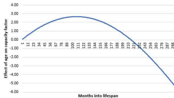
In Figure 2, the blue line is an example of the percentage point changes in capacity factor as the age of wind farm increases.
