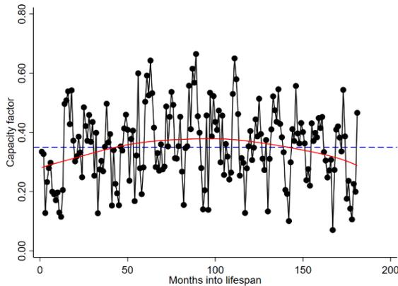
In Figure 1, the black, solid line with dots represents the actual, realized capacity factor of Barrow offshore wind farm. The horizontal blue and dashed line denotes the wind farm's average capacity factor based on currently available data. The red, solid line represents the smoothed, moving average of the capacity factor.
